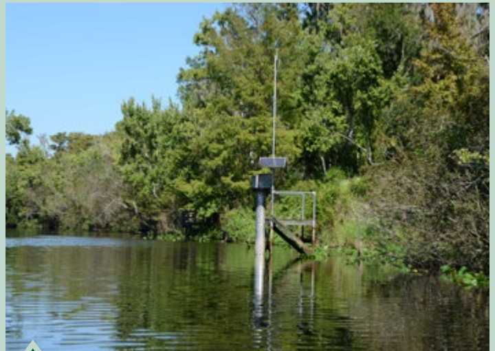
Hydrologic Monitoring Station on the Wekiva River
